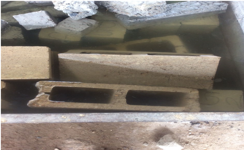
Figure 3.4 - 6-inch hollow sandcrete blocks immersed in water.
