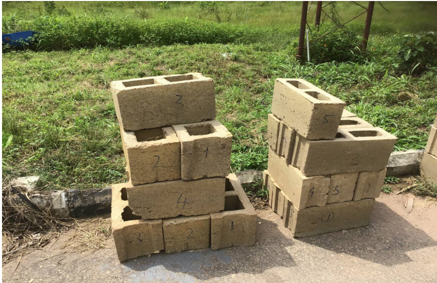
Figure 3.1- Hollow Sandcrete blocks from various Block industries.
