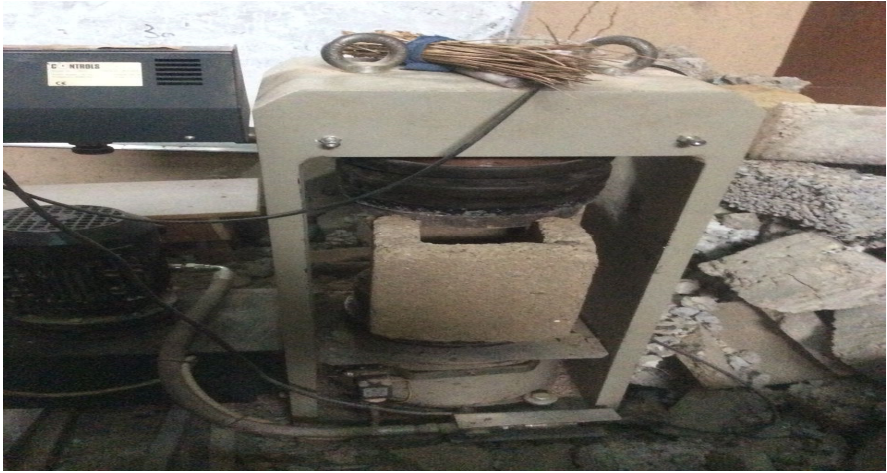
Figure 3.5 – Compressive strength test on hollow sandcrete block.
