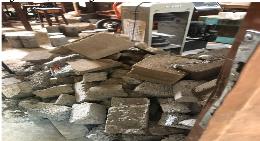
Figure 3: tested samples after crushing
