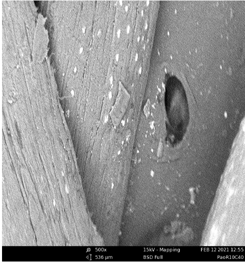
Plate 7: SEM of fractured surface from tensile measurement sample of P_{90}R_{10}C_{40} (filled with 40% CF)
