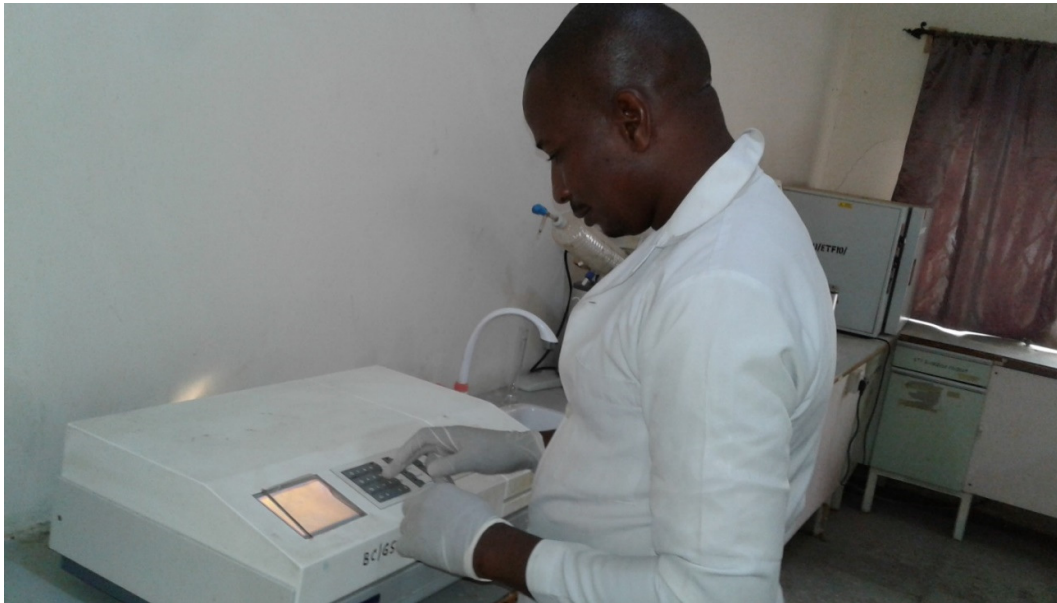
Plate 3: Measuring the absorbance of the MSW samples using Ultraviolet-Visible Spectrophotometer
