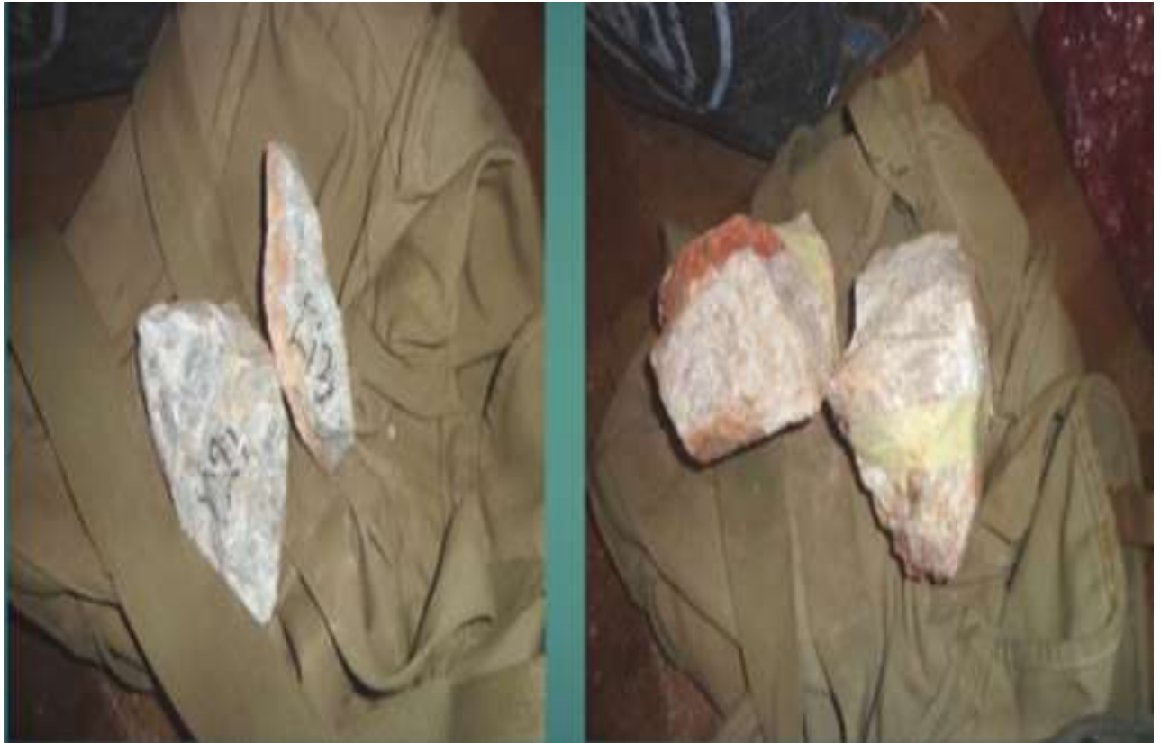
Plate 1: The Creamy/whitish variety that is Granular, Crystalline, sub-vitreous and consist of quartz
