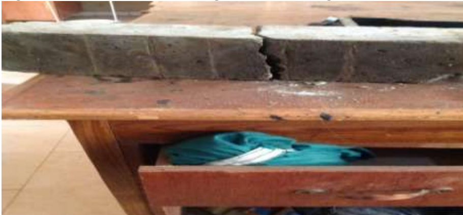
Fig. 4.1: Cracked Beam during flexural strength test
