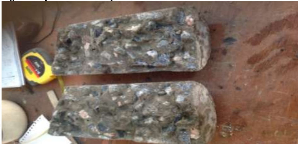
Fig. 4.7: Cylinder after Split Tensile Test
