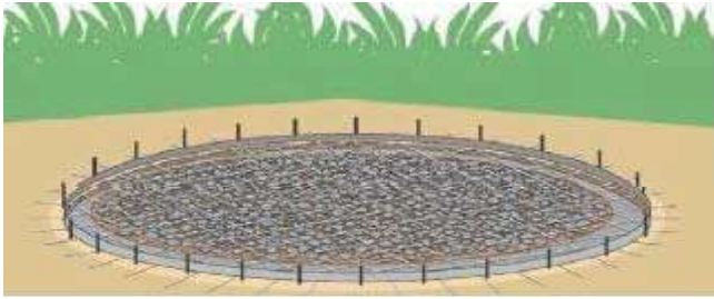
Fig 3.11: Plain GI strips and rebar ring comprise the base mold; a base course of gravel is laid
