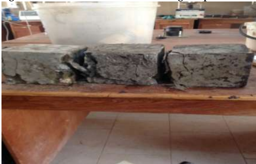
Fig. 4.5: crushed ferrocement cubes during compressive strength tests
