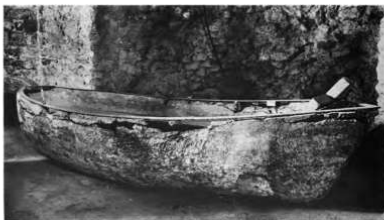
Figure 1.1: Lambot's original ferrocement boat built in 1848 now rests in the Brignoles Museum in France. (Brignoles Museum, France)
