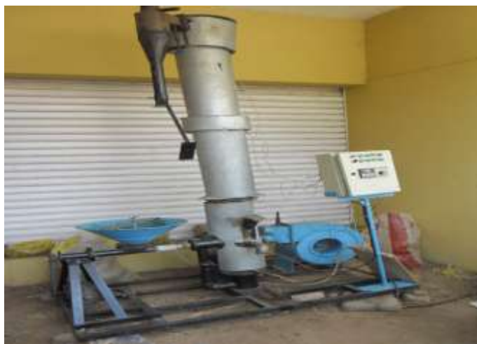
Fig. 1: Pictorial view of BFBC showing ITRU unit.
