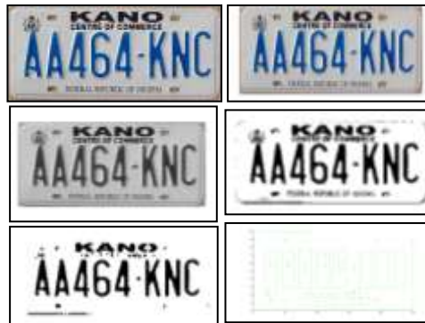
Figure 3: (Left to Right), License Plate, License Plate resized, License Plate in Grayscale, License Plate Binarized, License Plate Filtered, Blobs identified.
