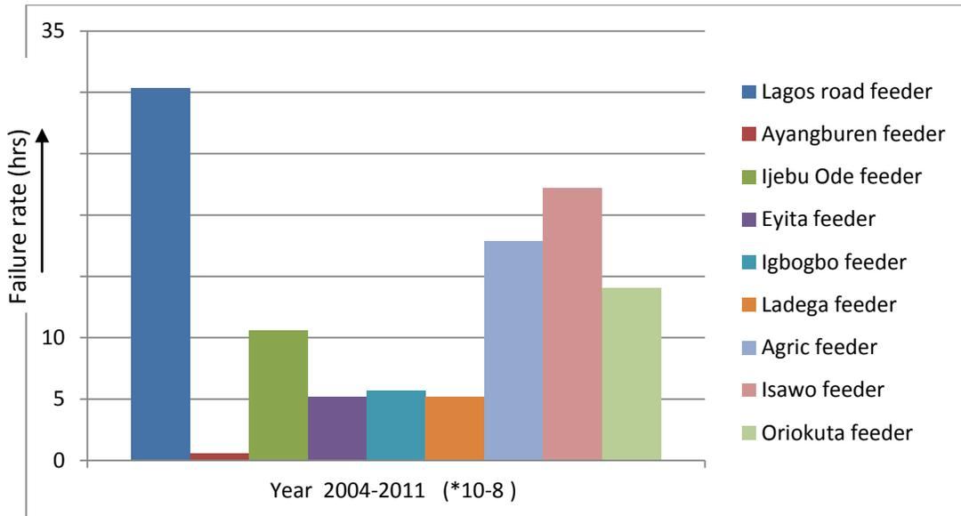
Figure 4.5: Reliability of the 11 kV Feeders (Year 2004-2011)
