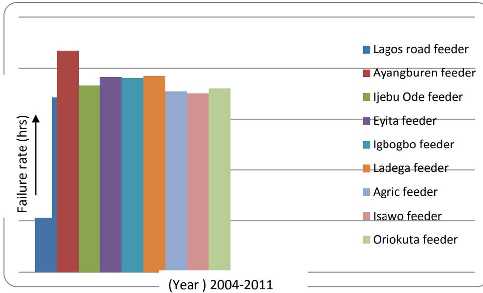
Figure 4.4: Failure Rate of 11 kV Lines Feeders (2004-2011)
