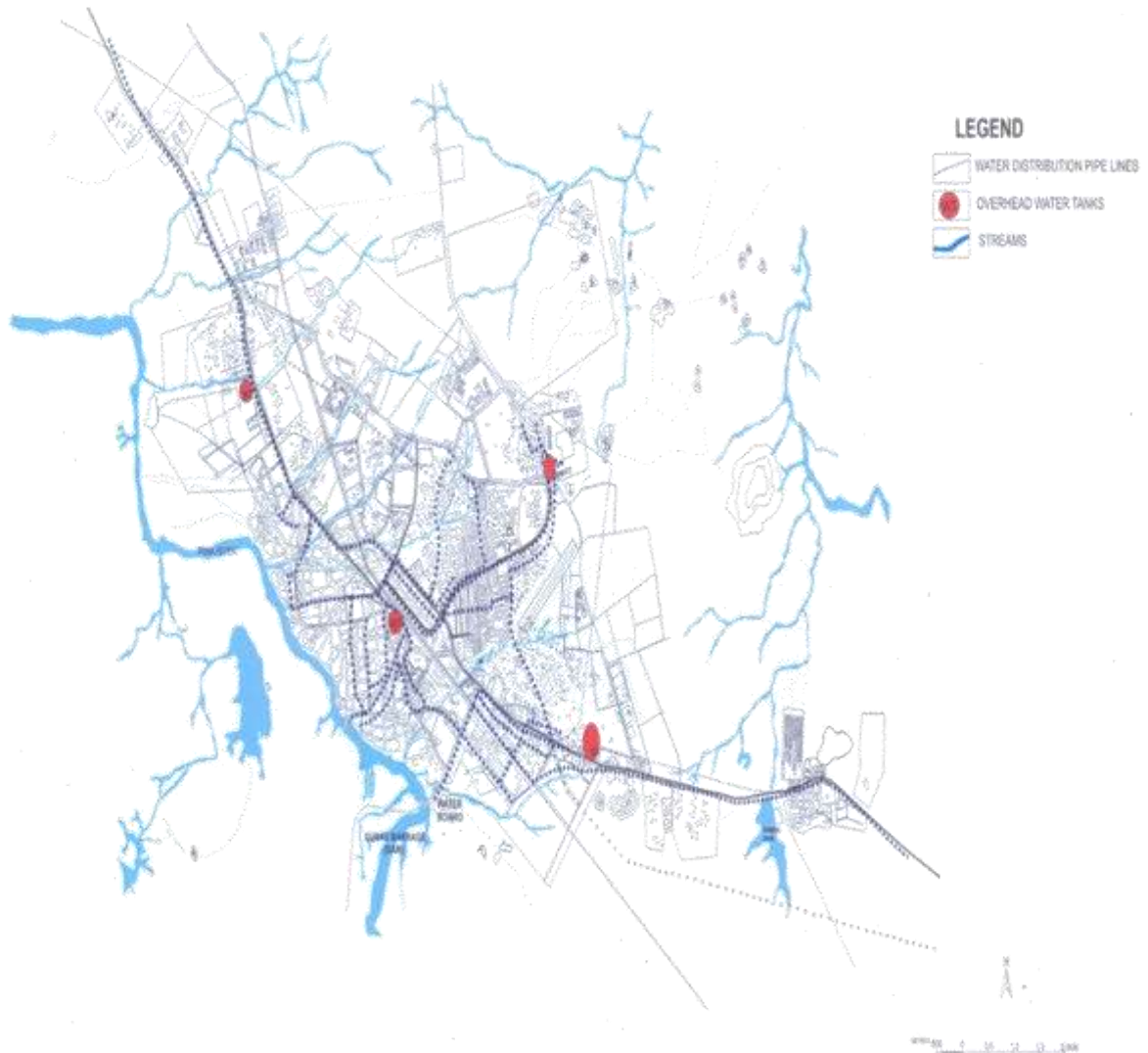
Fig. 2: Gusau Municipal Water Distribution Facilities
