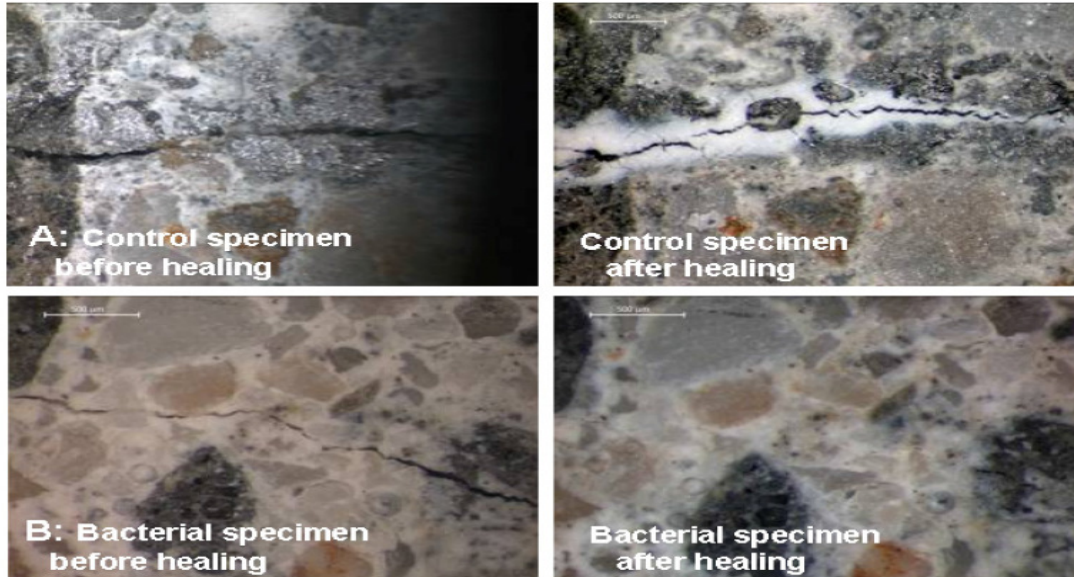
Figure 2. Light Microscopic Images (40 times Magnification) of Pre-cracked Control (A) and Bacterial (B) Concrete Specimen before (left) and after (Right) Healing (2 Weeks Submersion in Water). Mineral precipitation occurred predominantly near the crack rim in control but inside the crack in bacterial specimens. Efficient crack healing occurred in all six bacterial and two out of six control specimens.
