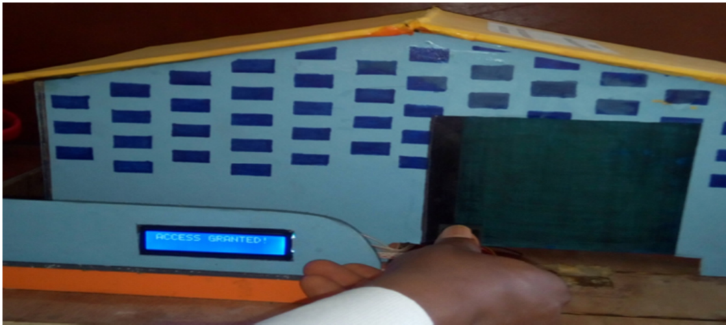
Figure 7: Snapshot showing access granted to a recognized fingerprint
