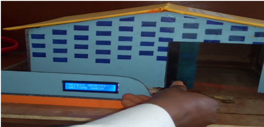
Figure 8: Snapshot showing door sliding open for the recognized user
