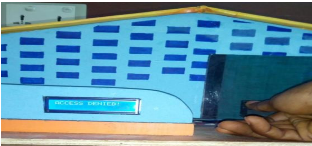
Figure 9: Snapshot showing access denied to an unrecognized fingerprint
