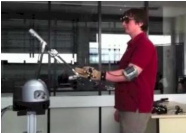
Fig 5: Haptic arm and cyber glove (Fillatreauet al., 2013)
