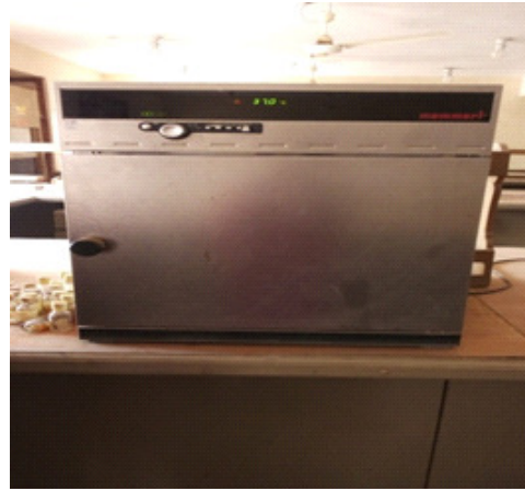
Plate B: Incubator closed at temperature of 37°C to allow formation of coliforms
