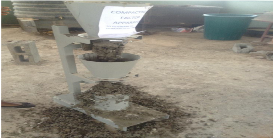
Figure 3.3 Compacting factor apparatus
