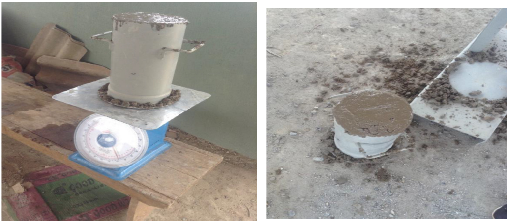
Figure 4.3 Compacted Concrete in Cylindrical Mould of Compacting Factor Apparatus
