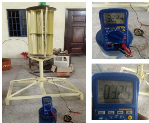
Figure 7: Voltage and current output at the maximum wind speed
