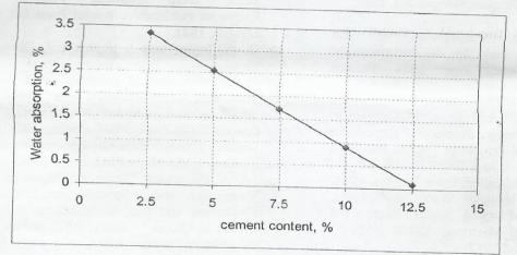
Effect of Cement Content on Water Absorption Fig.7.
