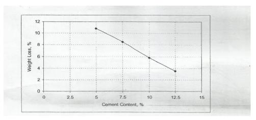
Fig.9 Effect of Cement Content on Durability
