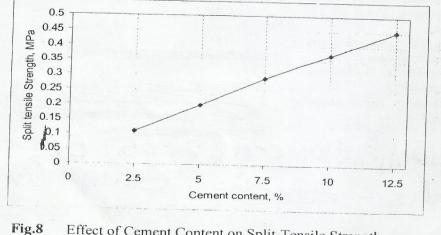
Effect of Cement Content on Split-Tensile Strength
