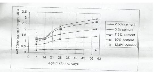
Effect of Age of Curing on Compressive Strength Fig. 6
