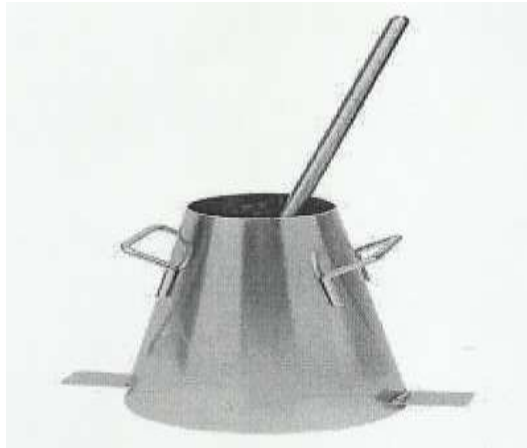
Fig 3.5: Slump Cone and Tamping Rod
