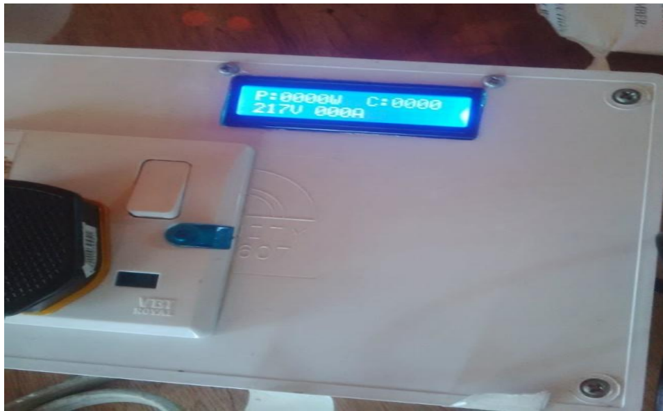
Figure 6: Constructed digital energy meter
